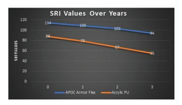
Figure 1. SRI values of Armor Flex and an acrylic PU roof coating over time.
